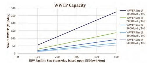
Figure 8. Typical wastewater treatment plant capacity if powered by 100 percent of electricity from a small energy-from-waste facility.
