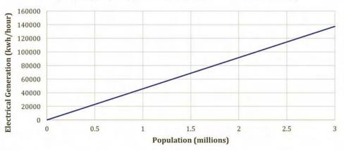
Figure 1. Typical energy from waste net electrical output as a function of population.
