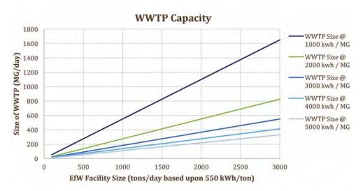
Figure 7. Typical wastewater treatment plant capacity if powered by 100 percent of electricity from a large energy-from-waste facility.
