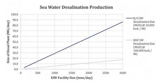
Figure 6. Water treatment capacity for seawater desalination if powered by 100 percent of electricity from an energy-from-waste facility.
