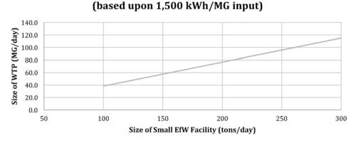
Figure 4. Water treatment capacity if powered by 100 percent of electricity from a small energy-from-waste facility.
