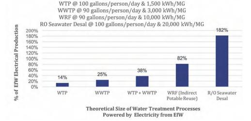
Figure 9. Range of sizes of water treatment processes that can be powered by a community's municipal solid waste.
