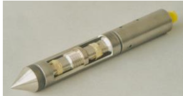
Figure 3 Electrical CPT(U) probe
