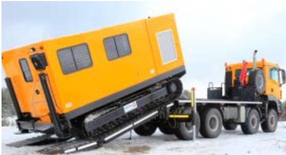
Figure 2 CPT-Crawler during mobilization
